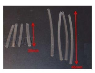
Slip the insulation over the neon lamp leads and with a hot air gun, shrink the tubing:
